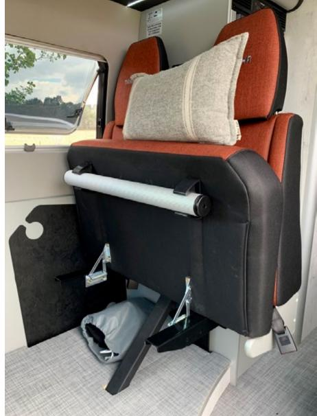
Both the dining and flip-up coffee tables are made of a new ultra-thin laminate that is super light yet very strong and rigid. It allows the dining table to be stored in a wafer-thin slot between the dinette seat and wall, while its leg clips neatly beneath the lift-up seat. What's in the bag? The magnetic blinds for the cab, that's what...
