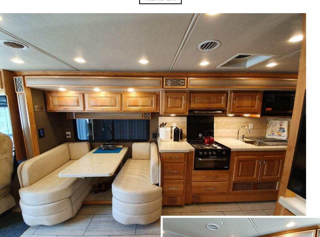
The kitchen has a three-burner gas stove and one electric hot plate and griller. There is an extraction fan above the stove, but it is too far back to be of any use and needs to be 300 mm further forward. The ceiling hatch open and the fan going is far more useful than the extractor fan. When not in use, the stove cover is a glass hinged top that is tempered glass, while for baking there is a convection microwave oven.
